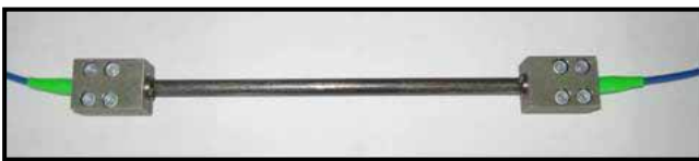
Figure 12. FBG crack meter ( large strain sensor)
