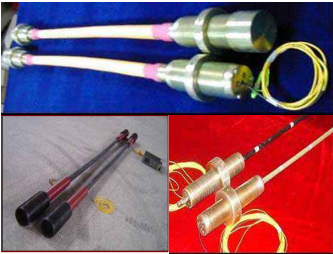
Figure 17. FBG-based smart cables
