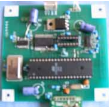
Figure 34. Top view of finished prototype wireless sensing unit
