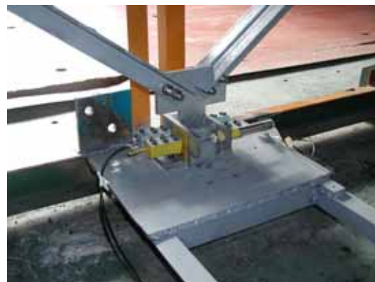
Figure 24. Integrated SMA damper/displacement transducer
