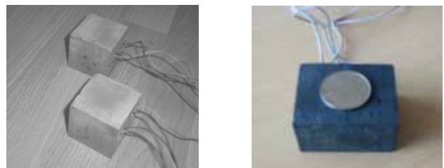
Figure 28. Photo of CSG sensor
