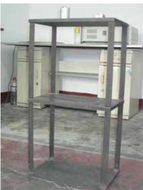
Figure 35. Photo of two-story steel frame structure model
