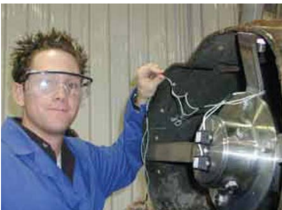
Masters student Chad Klowak installs accelerometers on top of the new SS rod that supports the Golden Boy. (Photo courtesy of ISIS Canada.)
