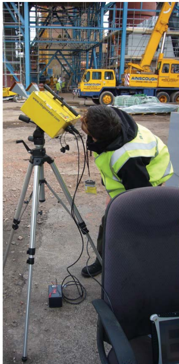
Figure 9a Aligning radar sensor
