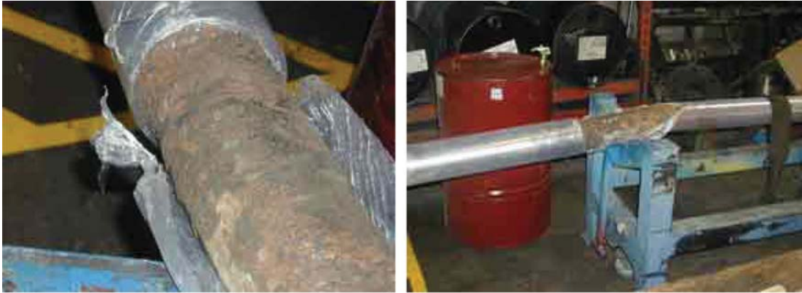
In places, the statue's steel support rod had lost up to 10 to 15 mm of its original 125-mm diameter. (Photos courtesy of ISIS Canada.)
