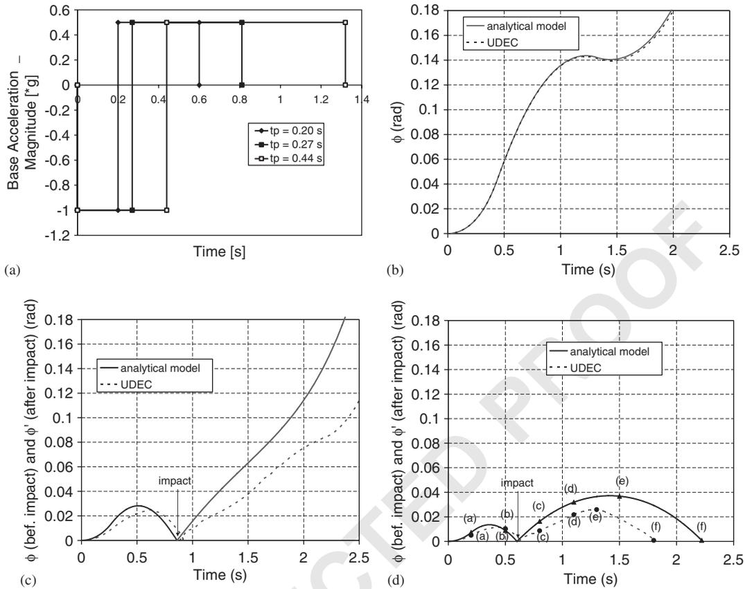
Figure 4. Applied impulses (a) and time histories of mechanism motion for  $a = 1.0g$  and  $t_p = 0.44$  (b),  $0.27$  (c), and  $0.20$  s (d).
