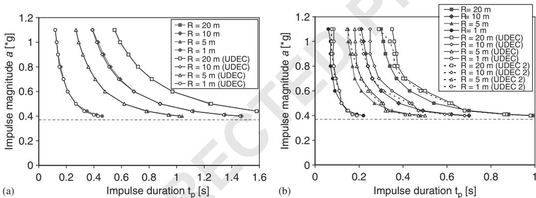
Figure 6. Effect of arch size on the failure domains for the first (a) and second (b) half cycles of motion. UDEC 2 = UDEC with reduced damping parameters ( $f_{min} = 0.05$  Hz and  $\zeta_{min} = 0.001\%$ ).
