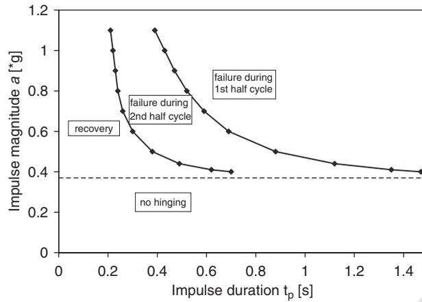
Figure 5. Failure domains of Oppenheim's arch in response to a step impulse function of duration,  $t_p$ , and magnitude,  $a$ , according to the analytical model.
