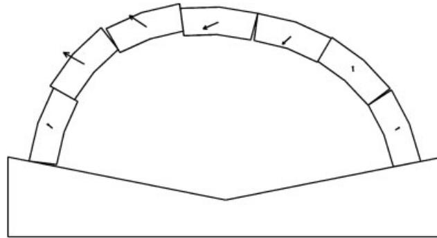
Figure 10. UDEC snapshot of Oppenheim's arch subjected to an impulse of magnitude  $a = 1.0g$  and duration  $t_p = 0.22$  s at time 1.29 s, with reduced Rayleigh damping ( $f_{\min} = 0.05$  Hz and  $\zeta_{\min} = 0.001\%$ ).
