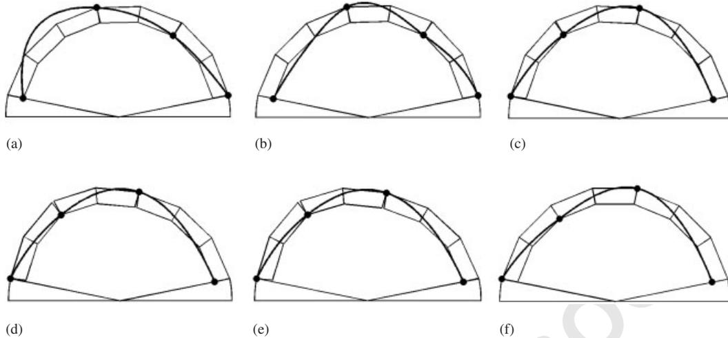
Figure 8. Arch hinge locations and thrust lines found using the analytical model for a step impulse of magnitude  $1.0g$  and duration  $0.20$  s at times: (a)  $0.20$  s; (b)  $0.50$  s; (c)  $0.80$  s; (d)  $1.10$  s; (e)  $1.50$  s; and (f)  $2.22$  s.
