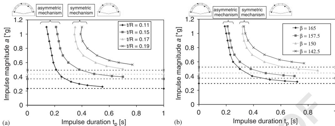
Figure 7. Effect of arch geometry on the failure domain (second half cycle,  $R = 10$  m).
