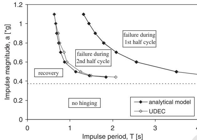
Figure 11. Failure domains of Oppenheim's arch in response to a single cycle sinusoidal impulse function of period,  $T$ , and magnitude,  $a$ .
