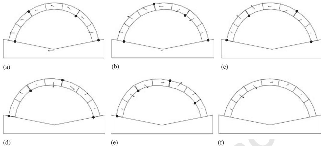
Figure 9. Arch hinge locations and block velocity vectors found using UDEC for a step impulse of magnitude  $1.0g$  and duration  $0.20\text{ s}$  at times: (a)  $0.20\text{ s}$ ; (b)  $0.50\text{ s}$ ; (c)  $0.80\text{ s}$ ; (d)  $1.10\text{ s}$ ; (e)  $1.30\text{ s}$ ; and (f)  $1.80\text{ s}$ .
