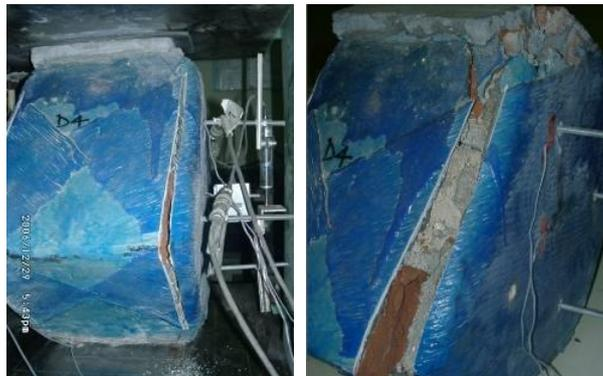
Figure 13: Damage of FRP retrofitted specimen C-1
