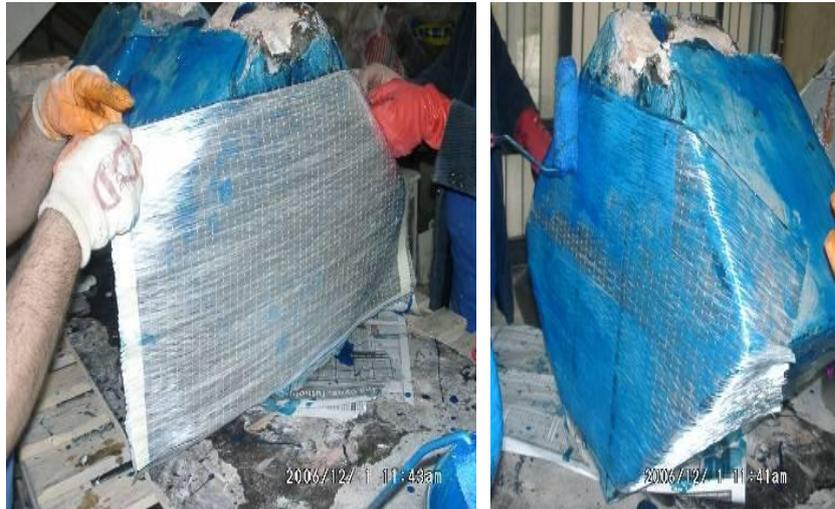
Figure 8: FRP application on specimens C-1 and C-2
