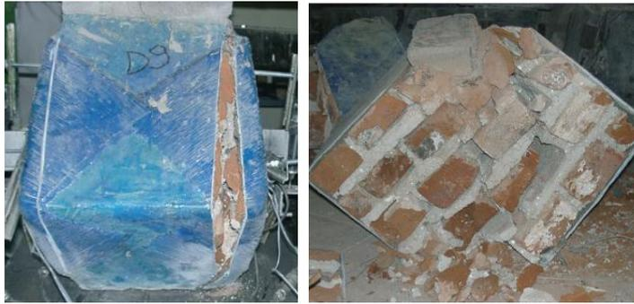
Figure 14: Damage of FRP retrofitted specimen C-2
