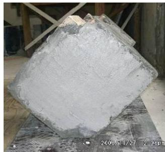
Figure 7: Plastered specimen
