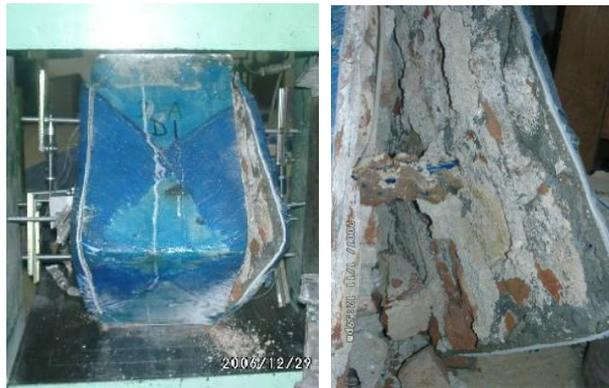
Figure 15: Damage of FRP retrofitted specimen D with FRP anchors
