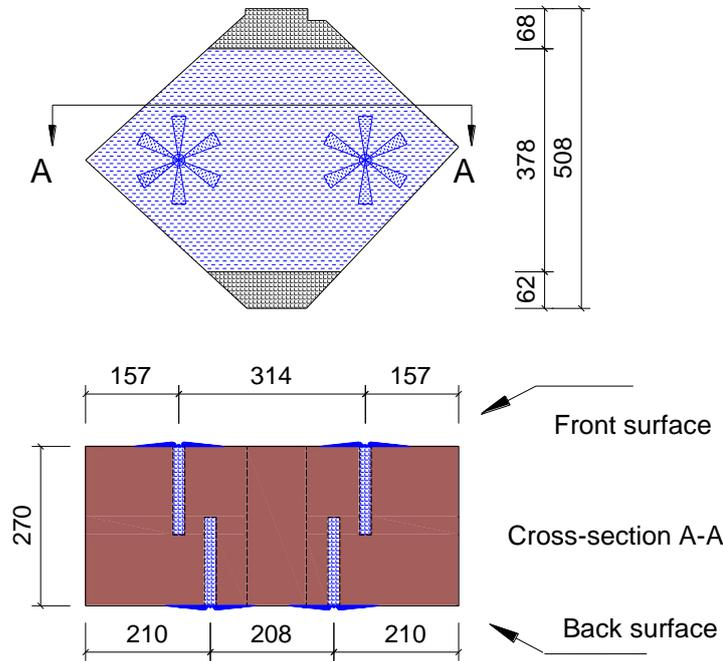
Figure 2: Type D specimen with FRP sheets anchored into the bricks, (units in mm)
