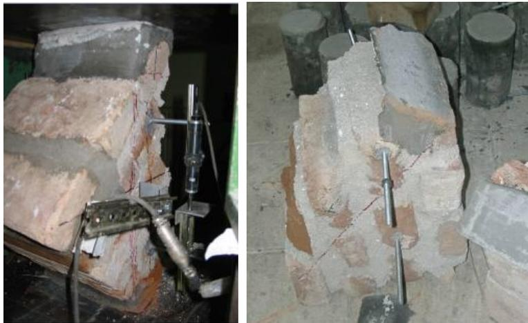
Figure 11: Damage of reference specimen A
