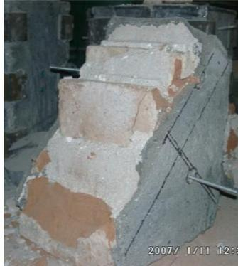
Figure 12: Damage of plastered specimen B
