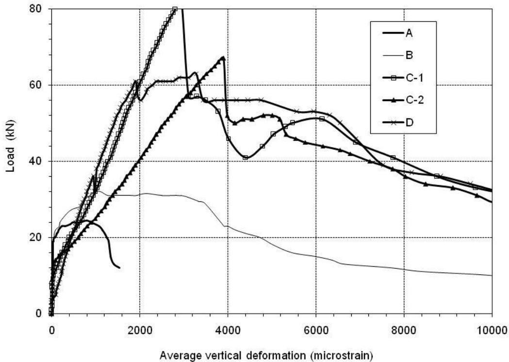
Figure 16: Load-average vertical strain relationships for all specimens (gauge length: 500 mm)
