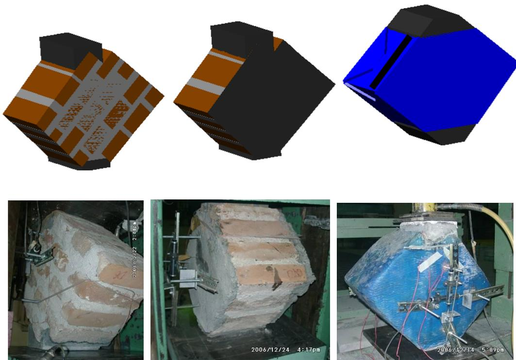
Figure 1: Reference (type A), plastered (type B) and retrofitted (type C) specimens
