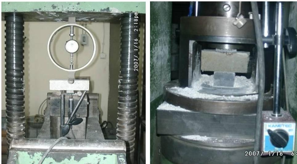
Figure 4: Tests for determination of mechanical characteristics of joint mortar
