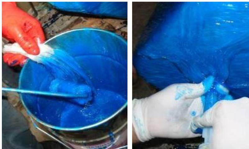
Figure 9: Application of glass FRP anchors into the retrofitted specimen D
