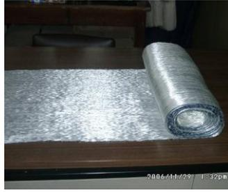
Figure 5: Glass FRP sheets to be used for retrofit of walls
