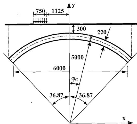
Figure 7. Geometry of the Bolton full scale model bridge (Melbourne and Walker 1989)
