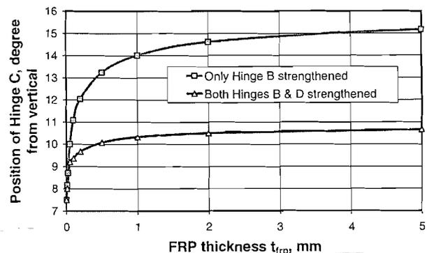
Figure 10. Effect of FRP thickness on hinge position
