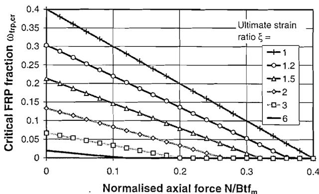
Figure 2. Minimum FRP fraction to prevent FRP rupture failure
