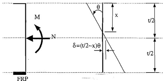
Figure 5. Virtual deformations at a hinge
