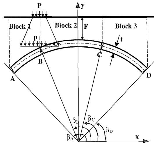
Figure 6. Load distribution and mechanism
