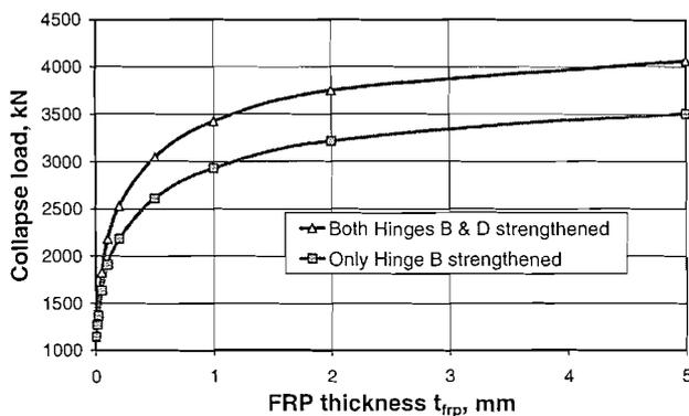
Figure 8. Effect of FRP thickness on the collapse load
