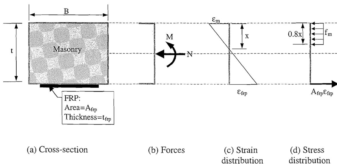
Figure 1. Ultimate state of an FRP strengthened rectangular masonry cross-section
