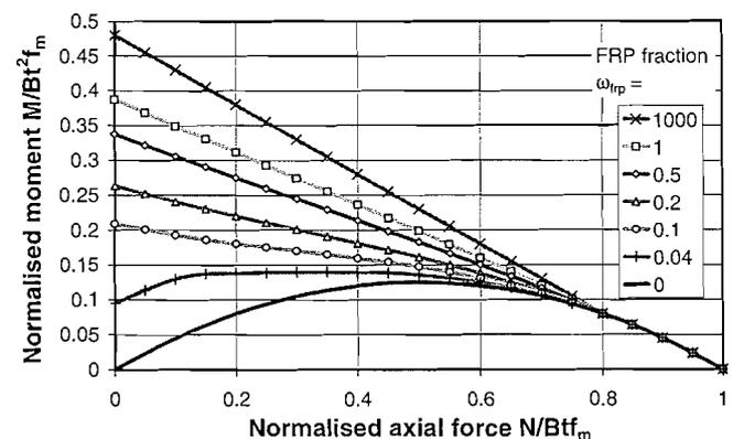
Figure 4.  $M-N$  relationship for various FRP fractions
