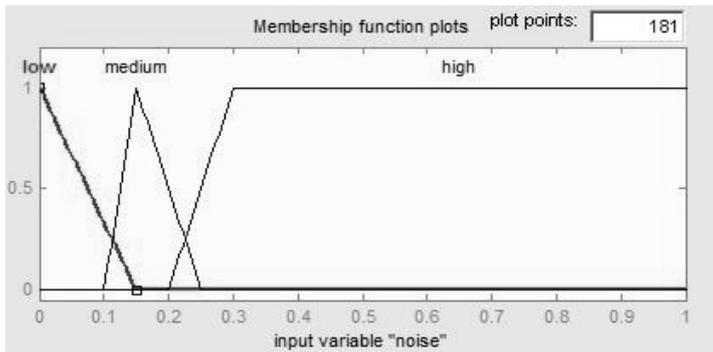
Figure 5. Membership functions for the noise-level
