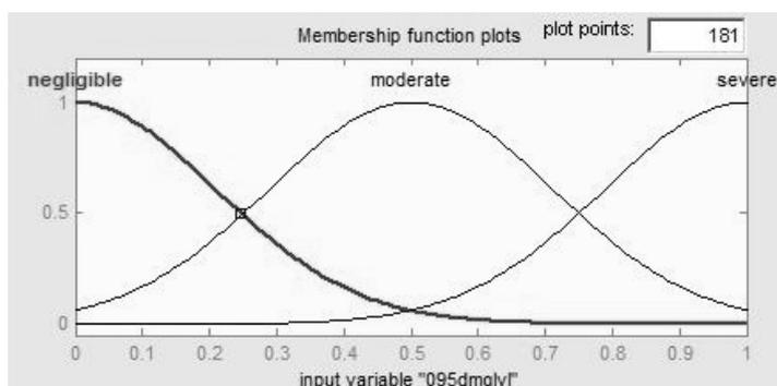
Figure 4. MATLAB™ depiction of damage level membership functions
