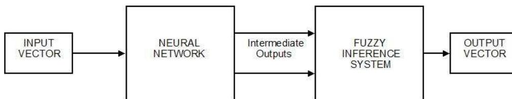
Figure 1. Flowchart depicting a typical serial neuro-fuzzy system
