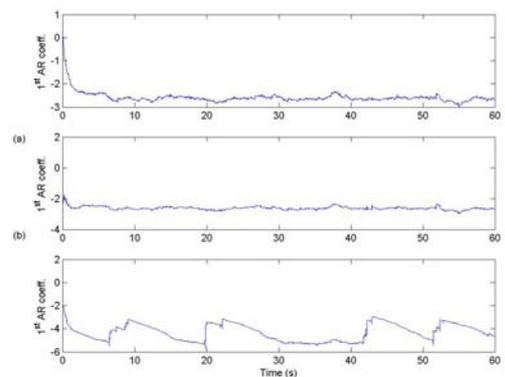
Figure 4. 1<sup>st</sup> AR coefficient for the 3DOF Bouc-Wen structure: (a) 1<sup>st</sup> storey, (b) 2<sup>nd</sup> storey, and (c) 3<sup>rd</sup> storey.
