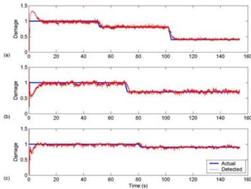
Figure 1. Stiffness detection in 3DOF linear model using forgetting factor: (a) 1<sup>st</sup> storey, (b) 2<sup>nd</sup> storey, and (c) 3<sup>rd</sup> storey.
