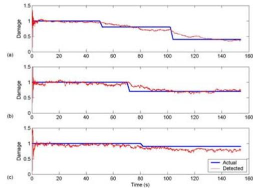
Figure 2. Stiffness detection in 3DOF linear model using Kalman filter: (a) 1<sup>st</sup> storey, (b) 2<sup>nd</sup> storey, and (c) 3<sup>rd</sup> storey.
