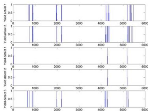
Figure 5. Detection of yielding in a 3DOF Bouc-Wen model: (a) actual 1<sup>st</sup> storey yield, (b) actual 2<sup>nd</sup> storey yield, (c) yield detected from 1<sup>st</sup> storey AR model, (d) yield detected from 2<sup>nd</sup> storey AR model, and (e) yield detected from 3<sup>rd</sup> storey AR model.
