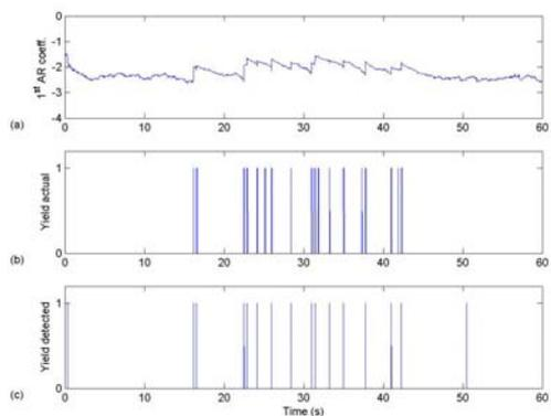
Figure 3. Yielding detection in a SDOF elastoplastic oscillator: (a) 1<sup>st</sup> AR coefficient, (b) actual yielding, and (c) detected yielding.
