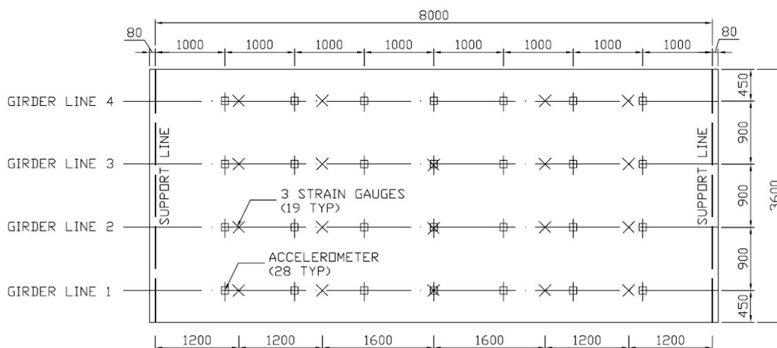
Figure 3. Plan view of bridge deck, showing the locations of accelerometers and strain gauge clusters (dimensions in mm).
