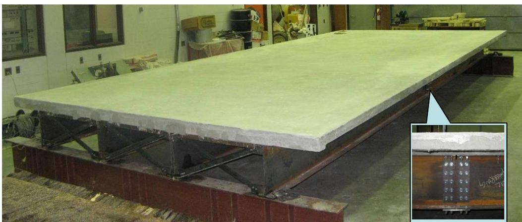
Figure 1. Slab on girder bridge superstructure built at 1/3<sup>rd</sup> scale (with inset showing the girder splice).
