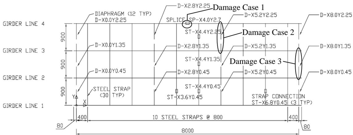
Figure 2. Plan view of the structural steel superstructure of the model showing splice and diaphragm locations (dimensions in mm).
