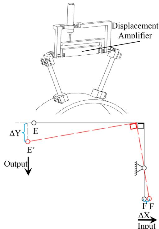
Figure.5 The sensing device with a displacement amplifier.
