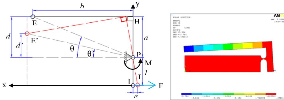
Figure.7 Analysis of amplification ratio.
