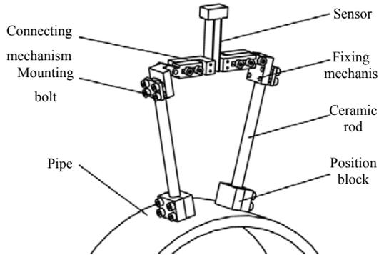
Figure.1 Designed Sensing Device.
