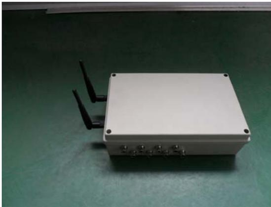
Figure 3. Wireless sensor node
