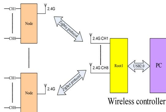
Figure 1. The system architecture of the acquisition system
