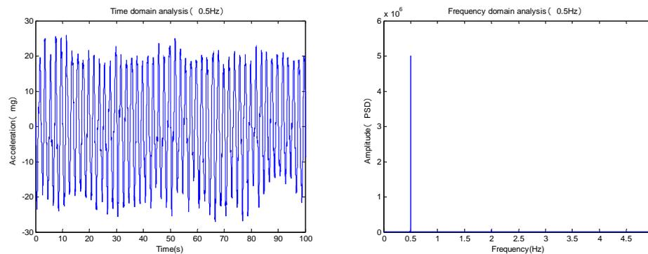
Figure 7. Time and frequency analysis of 0.5Hz
