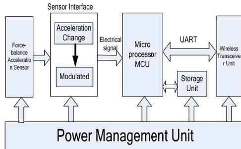
Figure 2. The low-frequency wireless acceleration sensor structure
