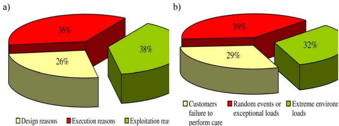
Fig. 1. Factors responsible for building failures: a - general classification, b – classification of exploitation reasons [1]
