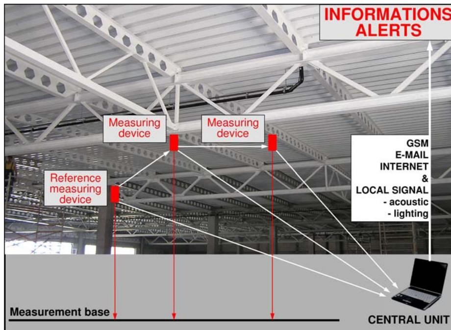
Fig. 3. Scheme of the WiSeNe monitoring system
