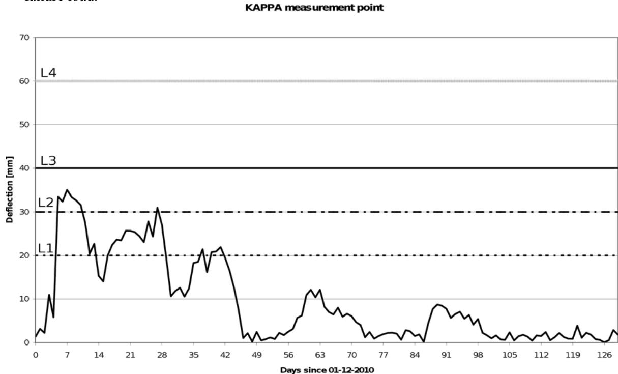
Fig. 6. Example of measured displacements for an industrial building
