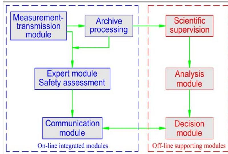
Fig. 7. General data flow diagram of WiSeNe<sup>MONIT</sup>
