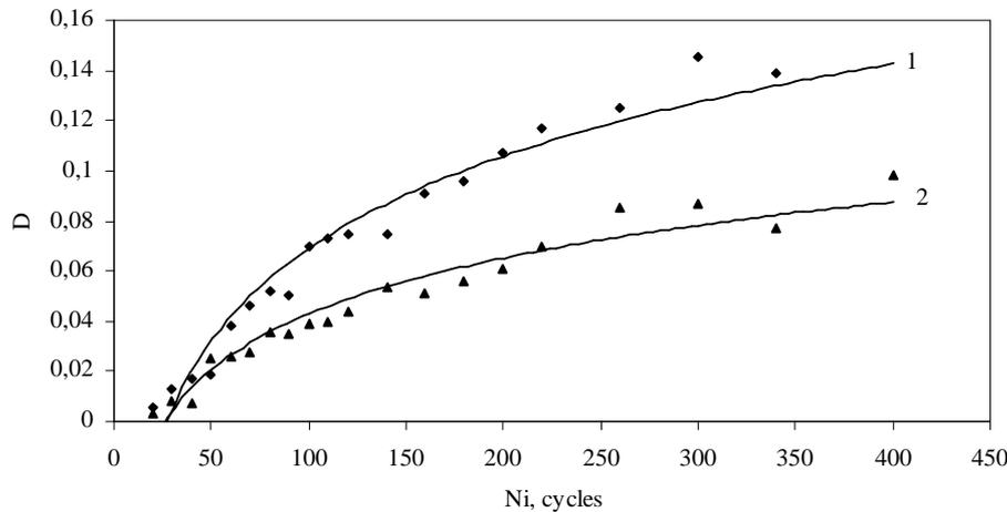
Figure 5. The evolution of damage parameter  $D$  for sensors of different sensitiveness: 1 – the maximum stress in the test portion of the sensor is equal to the  $\sigma_{\max}=280,0$  MPa; 2 – the maximum stress in the test portion of sensor is equal to the  $\sigma_{\max} = 240,0$  MPa.
