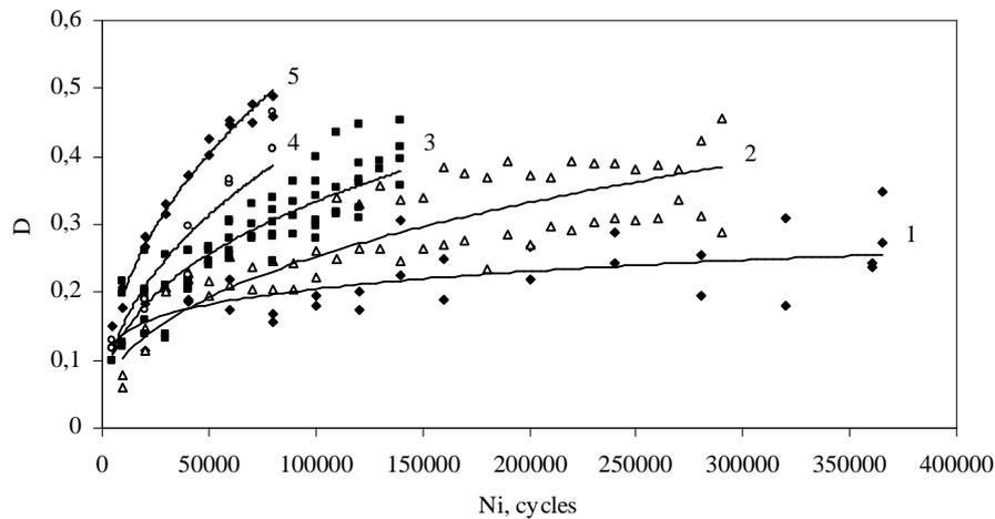
Figure 2. The evolution of damage parameter  $D$  on the surface of alclad aluminum alloy under cyclic loading: 1)  $\sigma_{\max}=76,9$  MPa; 2)  $\sigma_{\max}=81,7$  MPa; 3)  $\sigma_{\max}=96,2$  MPa; 4)  $\sigma_{\max}=115,4$  MPa; 5)  $\sigma_{\max}=134,6$  MPa.
