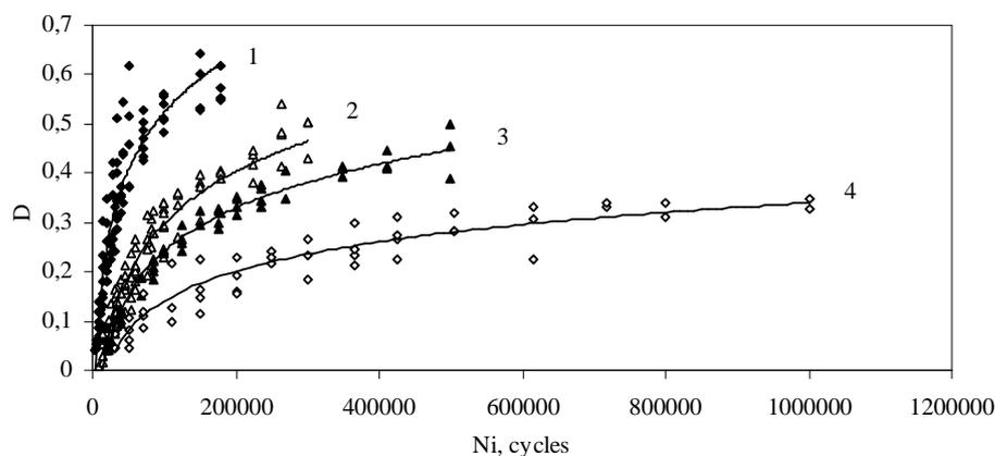
Figure 3. Evolution of damage parameter  $D$  during asymmetrical loading process under stress ratio: 1)  $R=0,2$ ; 2)  $R=0,42$ ; 3)  $R=0,5$ ; 4)  $R=0,6$ .
