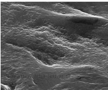
Figure 1. Extrusion/intrusion structure of the cyclically deformed aluminium.
