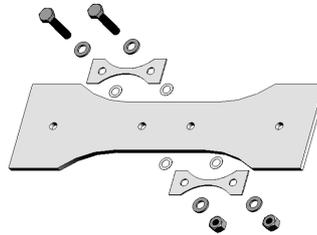
Figure 4. 3D image of the sensor attachment to the specimen for fatigue test
