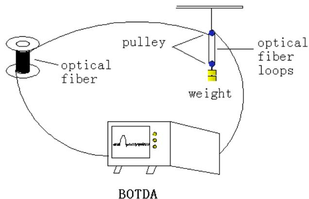
Figure 3. set up of static load experiment.
