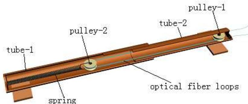
Figure 1. Packaging structure of fiber optical Brillouin displacement sensor.
