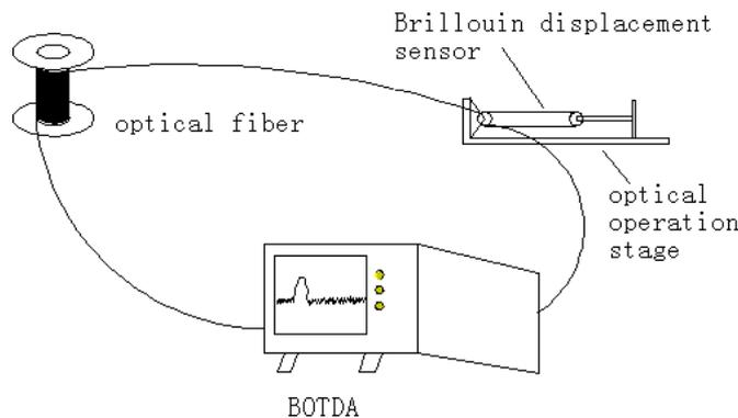
Figure 4. set up of displacement calibrating experiment.
