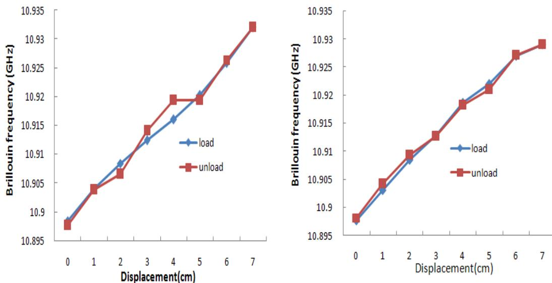
Figure 6.Brillouin frequency result of load cycle 1<sup>st</sup>. Figure 7.Brillouin frequency result of load cycle 2<sup>nd</sup>.
