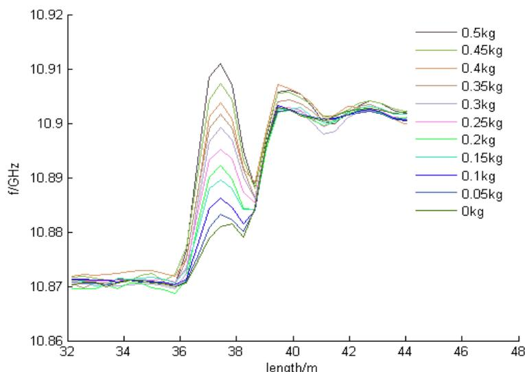
Figure 5. Brillouin frequency result of static load experiment.
