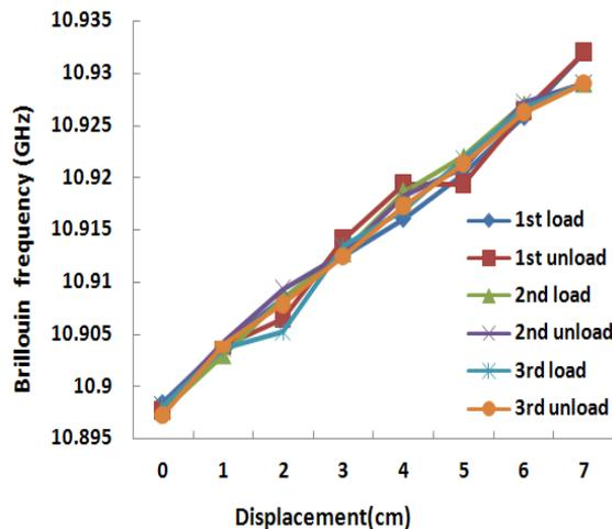
Figure 8. Brillouin frequency result of load cycle 3<sup>rd</sup>.
