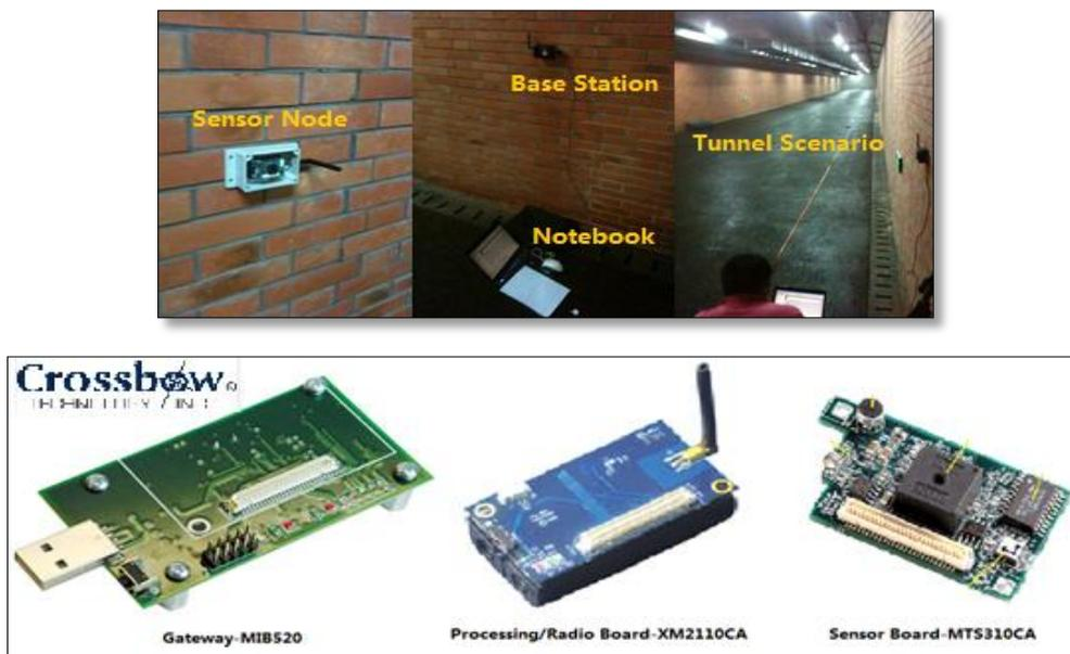
Figure 2. Situ-test, gateway and sensor photos (sensor board photo of provided by Crossbow Inc.)
